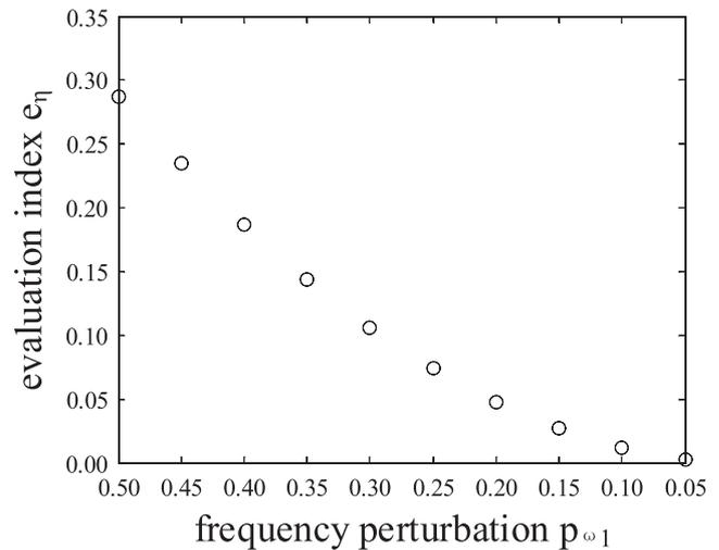
Fig. 4. Evaluation index corresponding to different frequency perturbation range.
