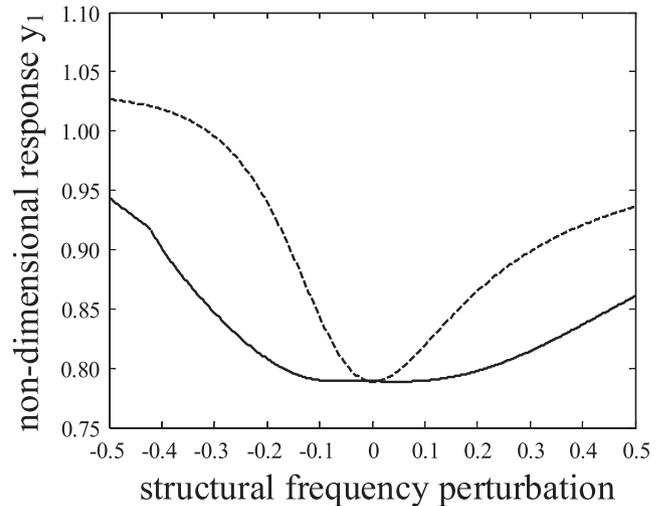
Fig. 6. Contrast of non-dimensional response of structure attached with linear TMD (—) and nonlinear TMD (---).
