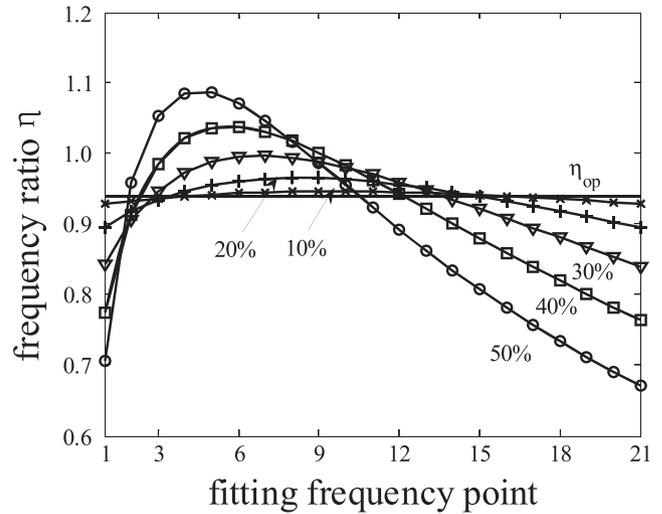
Fig. 3. Fitting frequency ratio corresponding to different frequency perturbation range.
