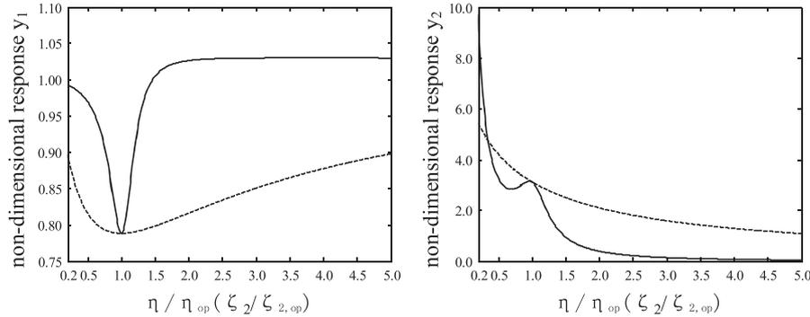
Fig. 2. Effect of perturbation of frequency and damping ratio on non-dimensional response of (a) structure and (b) linear TMD,  $m_1 = 1$ ,  $\zeta_1 = 0.05$ ,  $\mu = 0.03$ , frequency ratio perturbation —, damping ratio perturbation - -.
