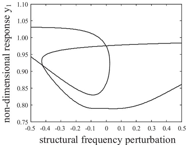
Fig. 5. Multiple steady state response of structure attached with nonlinear TMD.
