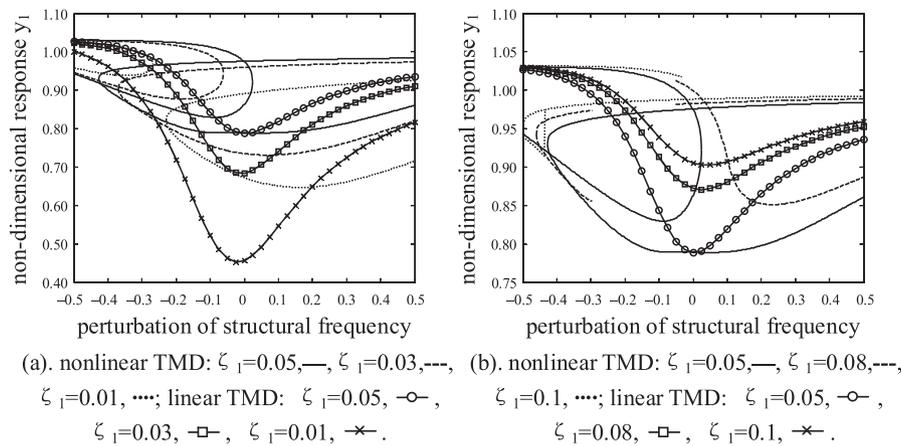
Fig. 8. Sensitivity of linear and nonlinear TMD's performance for vibration suppression of structure to (a) decreased and (b) increased structural damping ratio,  $m_1 = 1$ ,  $\mu = 0.03$ .
