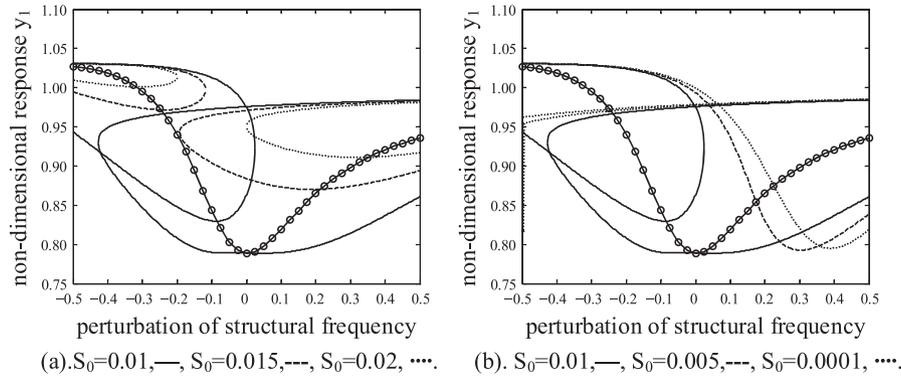
Fig. 7. Sensitivity of nonlinear TMD's performance for vibration suppression of structure to (a) increase and (b) decreased excitation intensity,  $m_1 = 1$ ,  $\mu = 0.03$ ,  $\zeta_1 = 0.05$ , linear TMD:  $\text{---}\bigcirc\text{---}$ .
