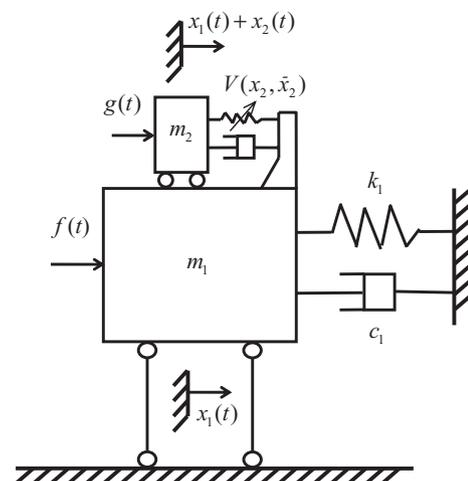
Fig. 1. Schematic model of the structure -nonlinear TMD system.
